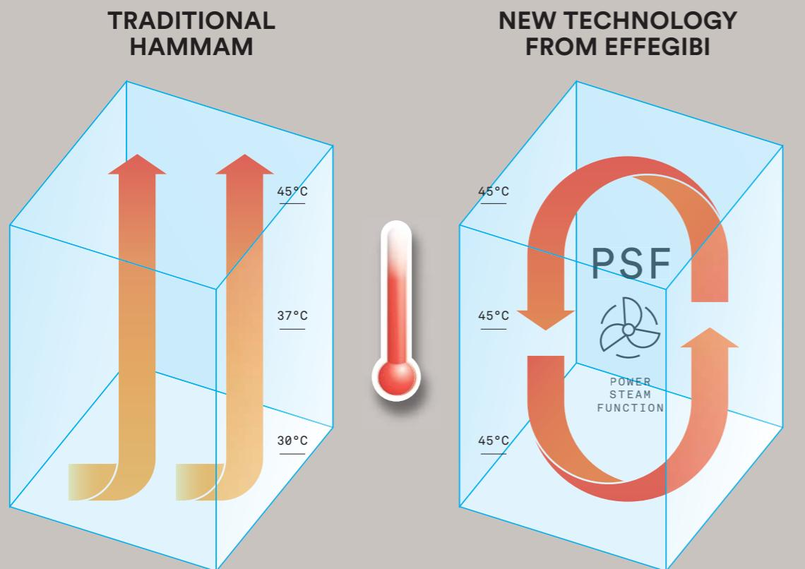
The innovative ventilation management system minimises temperature layering inside the cubicle.
